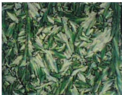
Fig. 11. Fan-broken texture (magnification \times 210 ) detected in the induced S_{C^*} at T = 73^\circ\text{C} .
